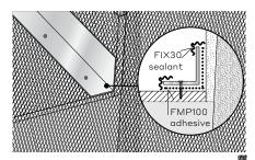
\*The thickness of the MULTIPANEL upstand is dependant on the support structure behind it. A minimum 16mm MULTIPANEL upstand is required when wall frame spacings are at 450mm centres. If adhering MULTIPANEL upstands to a solid surface, any thickness MULTIPANEL can be used to suit the overall wall finish.
