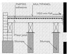
Outer edge of panel to extend over the edge of the balcony or into a box gutter.
